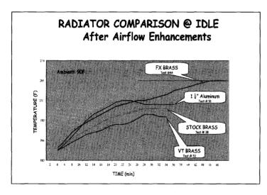
were better than stock on the highway, but even there stock was acceptable. Although the results were not necessarily what we expected, it emphasized the real importance of maximizing airflow and the value of scientific testing over anecdotal conclusions.
